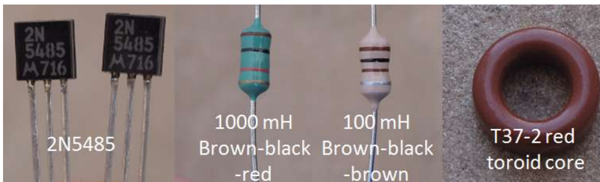
Figure 35. JFET transistors, 1000/100 mH molded chokes, and VFO T37-2 core
