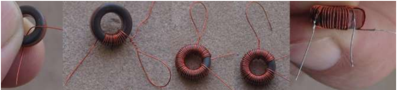
Figure 38. VFO coil L9. 40m version shown.
