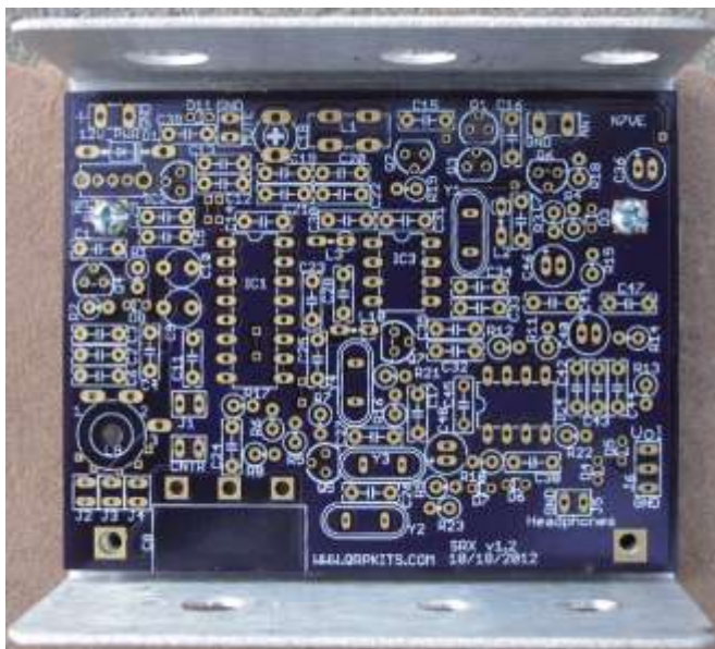
Figure 7. Temporarily mount PCB in chassis
