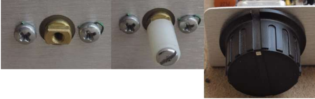
Figure 55. Installation of main tuning hardware
