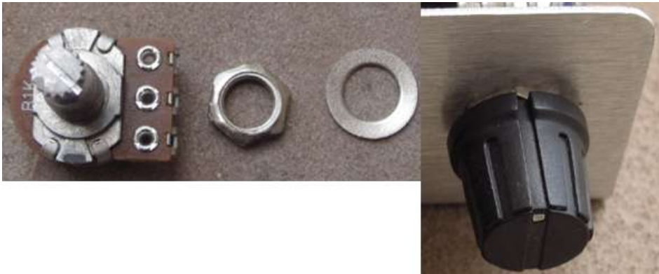
Figure 58. Volume control pot mounted to the front panel
