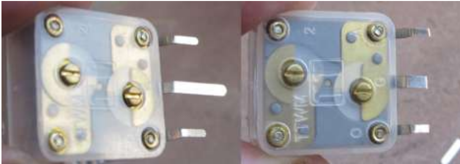
Figure 8. Prepare the leads of the main tuning capacitor
