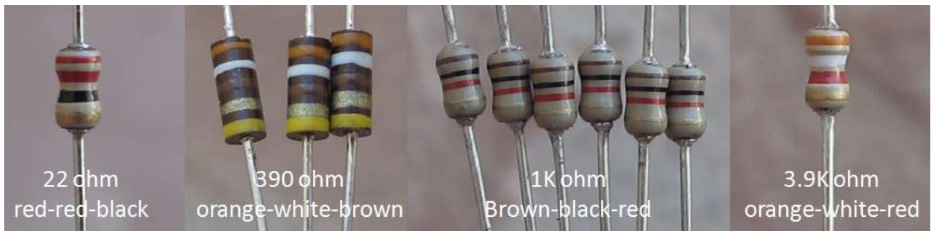
Figure 15. Resistors installed in this section
