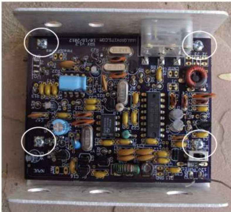
Figure 54. Mount PCB in case using four 4-40 screws
