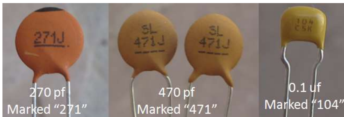
Figure 23. Capacitor markings for the first set of capacitors installed
