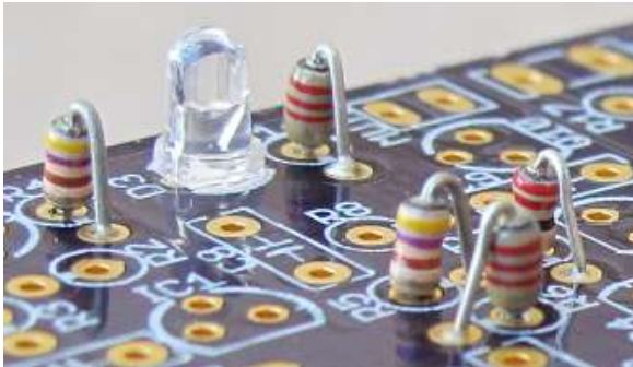
Figure 13. Resistors are mounted vertically, with short leads, body on the circle, close to the PCB
