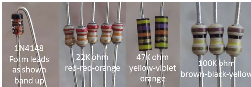
Figure 18. Picture of resistors installed in this section
