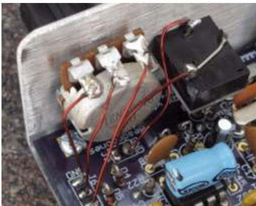
Figure 57. Wiring of the headphone jack and volume control to the PCB
