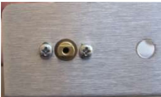
Figure 9. Mount the main tuning cap to the front panel
