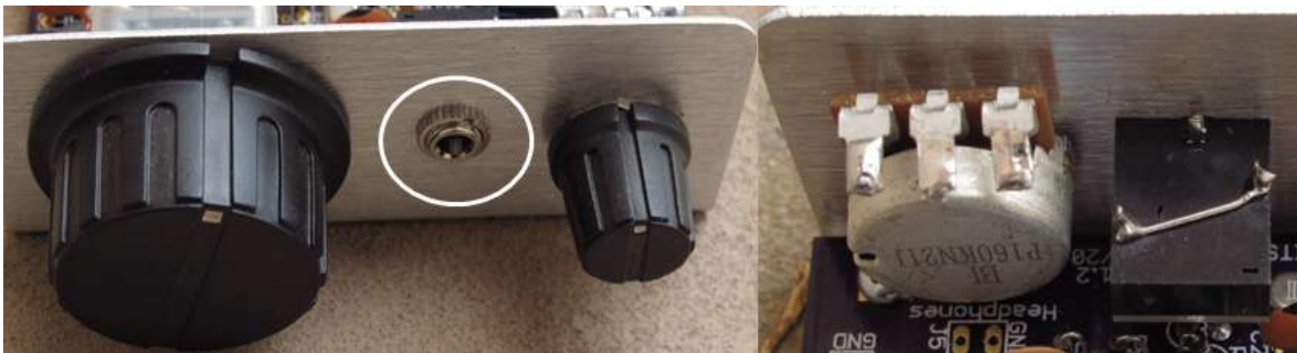
Figure 56. Mounting of the headphone jack
