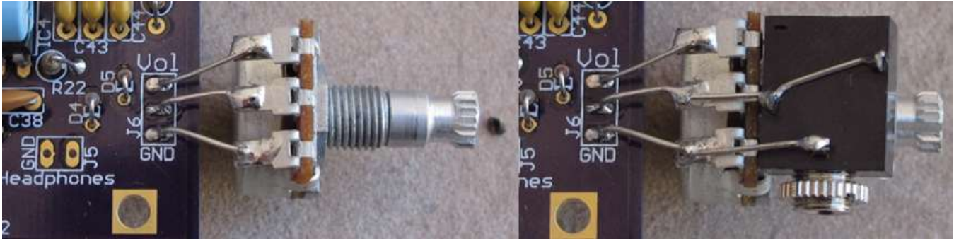
Figure 48. Temporary installation of volume pot and headphone jack for testing
