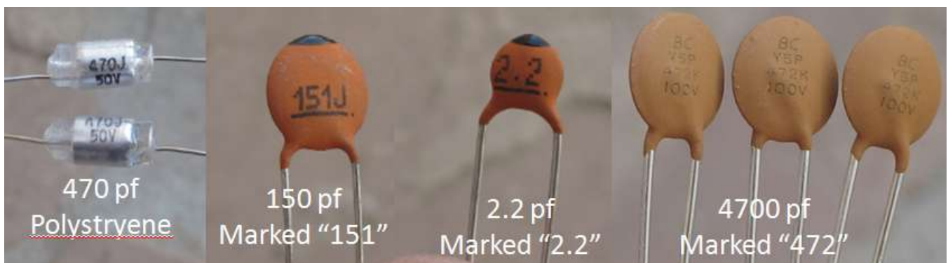
Figure 26. Markings on the second set of capacitors to be installed
