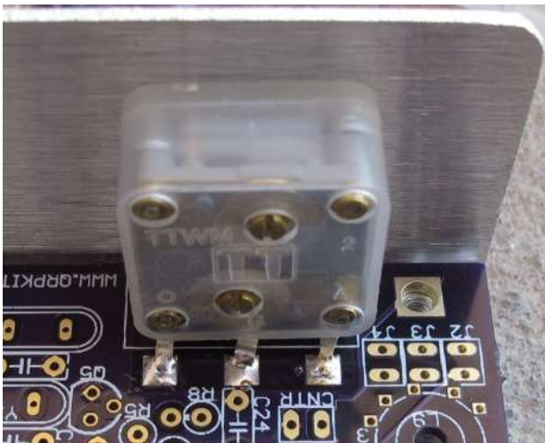
Figure 10. Solder main tuning cap leads from the top side of the PCB
