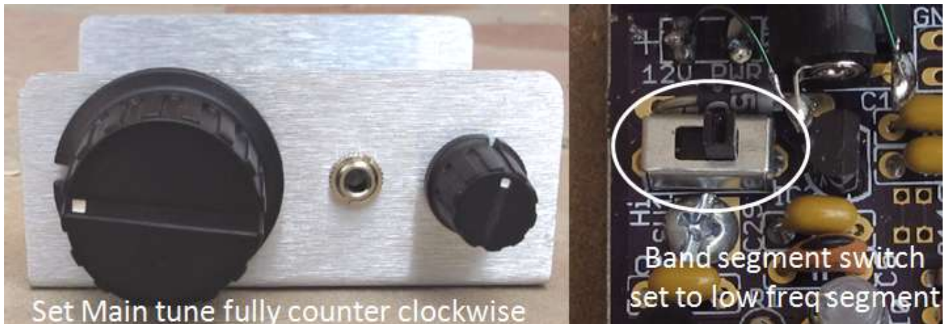
Figure 62. Picture main tune set to the lowest frequency, band segment switch set to low freq
